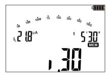
The value of leakage current  $I_L$  measured in time t=5'30'. Symbol  $J_{\rm s}$  indicates the selected time interval, in which the leakage current value was recorded.
